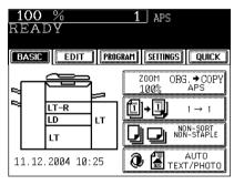
If the automatic density mode is not selected, press the (MANUAL) key, then press the (AUTO) key on the next screen.
